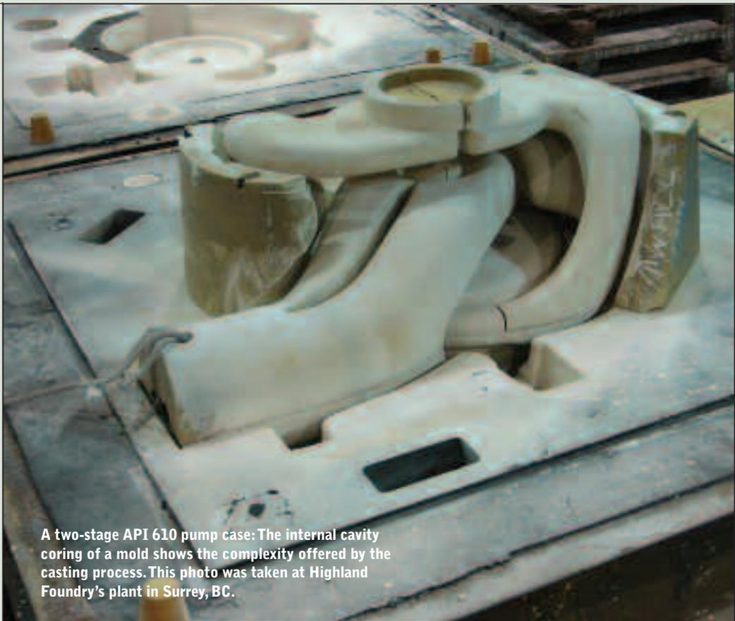
**A two-stage API 610 pump case: The internal cavity coring of a mold shows the complexity offered by the casting process. This photo was taken at Highland Foundry’s plant in Surrey, BC.**
