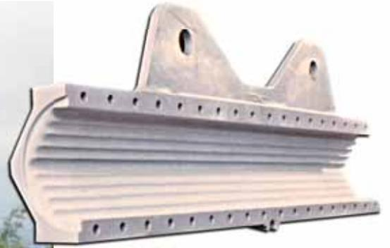
cables. The cast clamp was made out of ASTM A148 grade 115-95 steel. Each casting was half a clamp, measured 92 in. long and weighed 1,700 lbs.
